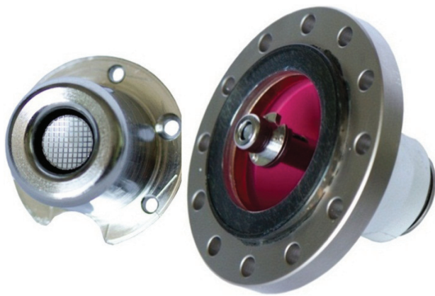
Figure 3: Photo of an injector with a mask on the cathode.
