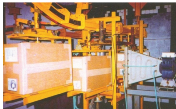
Figure 2: Irradiated devices on conveyor in the accelerator complex of JSC "MRTI RAS".
