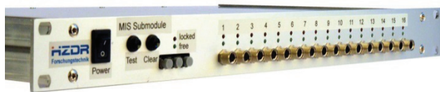
Figure 3: Fast logic interlock system, front view of sub module.
