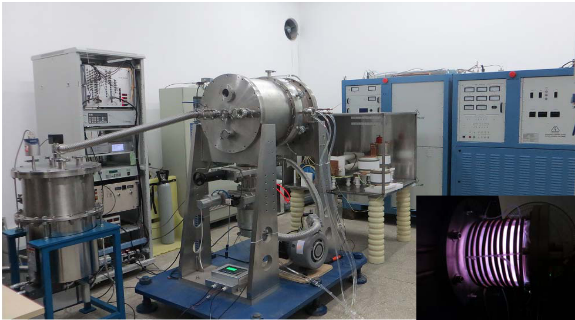
Figure 4: The integrated system with the small cylinder. At right and bottom is the photo of plasma ignition.
