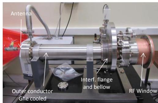
Figure 5: RF Coupler prototype assembled for leak tests in clean room.
