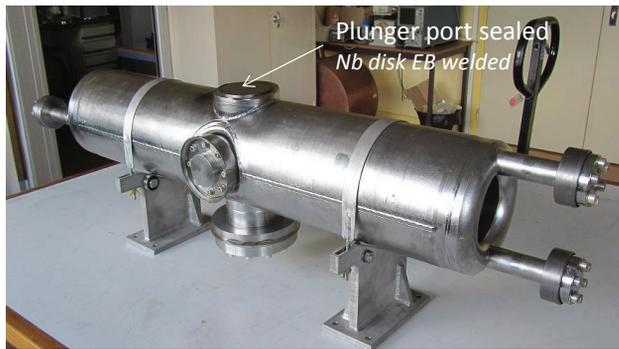
Figure 2: HWR prototype after modification (without helium tank).
