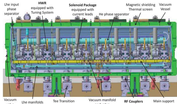
Figure 1: General layout of the IFMIF-LIPAc SRF Linac.
