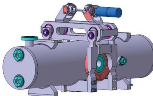
Figure 4: Mechanical design of the low-beta HWR, tuned by beam noses compression.
