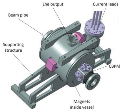
Figure 6: Detailed design of the Solenoid Packages.
