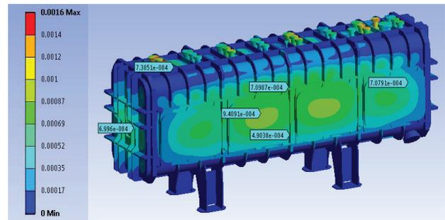
Figure 7: Mechanical deformation of the vacuum tank under operation conditions.
