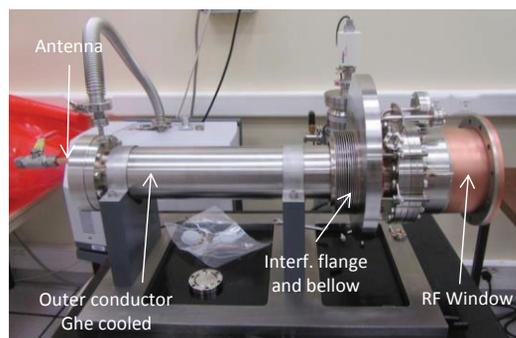
Figure 5: RF Coupler prototype assembled for leak tests in clean room.
