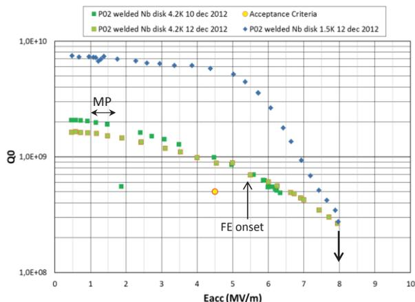
Figure 3: Cold tests results of HWR prototype:  $Q_0$  vs  $E_{acc}$ .
