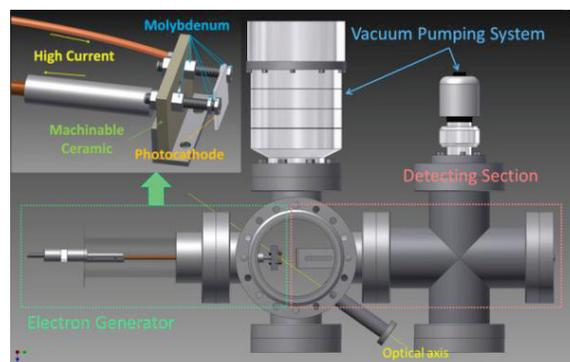
Figure 1: Equipment used to measure the quantum efficiency.
