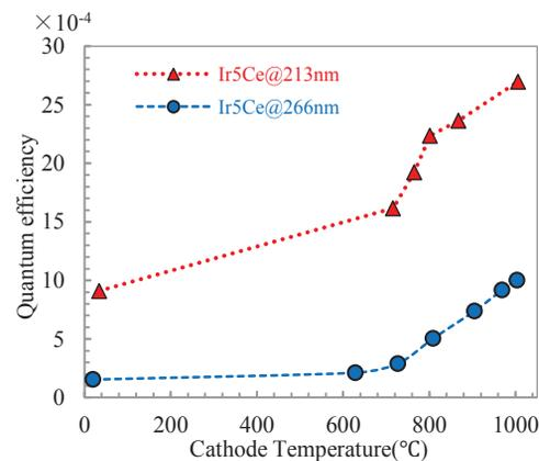
Figure 4: The QE of the Ir<sub>5</sub>Ce photocathode as functions of the surface temperatures.
