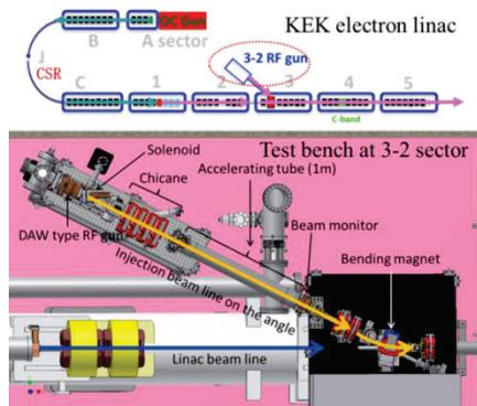
Figure 6: Figures of the existing beam line and the test bench at the 3-2 sector in KEK.
