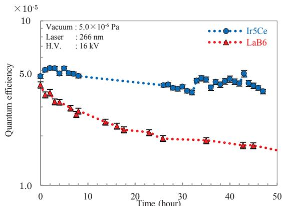
Figure 5: The dependence of QE on the irradiation time.
