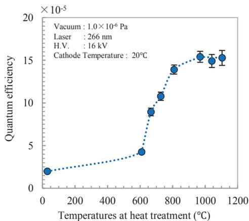
Figure 3: The QE of the Ir<sub>5</sub>Ce photocathode as a function of the heat-treatment temperatures.
