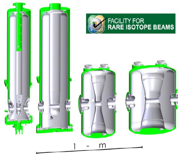
Figure 1: FRIB resonators. From left:  $\beta_0=0.041$  and  $0.085$  QWRs,  $\beta_0=0.29$  and  $0.53$  HWRs.
