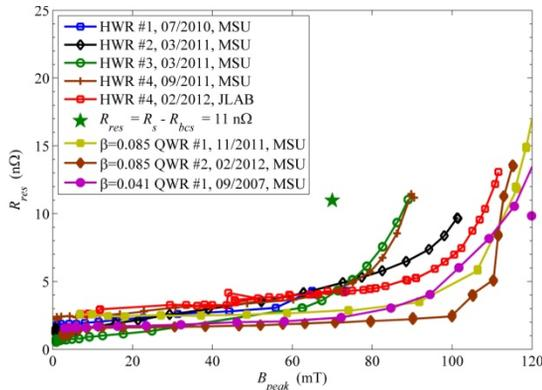
Figure 4: Residual surface resistance at 2K of  $\beta_0=0.041$  QWR,  $\beta_0=0.085$  QWR and  $\beta_0=0.53$  HWR prototypes.
