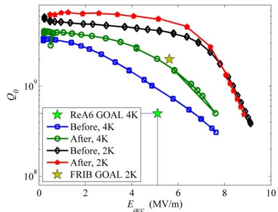
Figure 2: ReA3,  $\beta_0=0.085$  QWR prototype Q vs.  $E_a$  at 2K and 4.2K, before and after 120°C baking.
