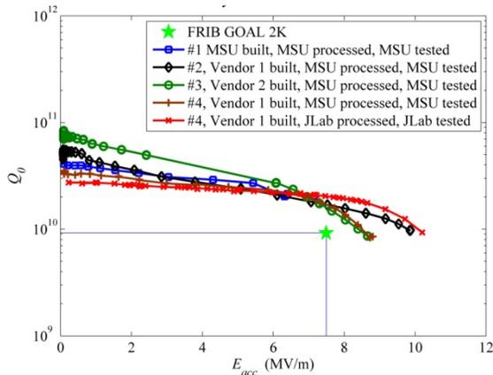
Figure 3: Performance of the  $\beta_0=0.53$  HWR prototypes processed and tested at MSU and JLAB.
