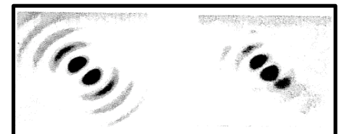
TEM 10 -like mode simulated (left) and imaged (right) at BNL ATF
