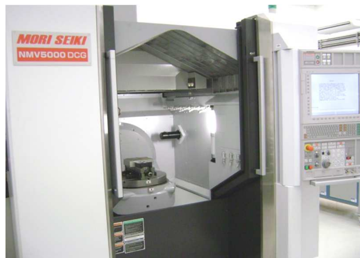
5 axis machining center Precision: 0.003 mm
