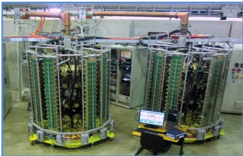
RF system using solid state amplifiers at 476 MHz developed in collaboration with Soleil.
