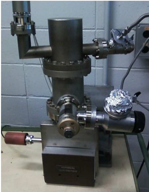
Ion pump in conventional set-up
