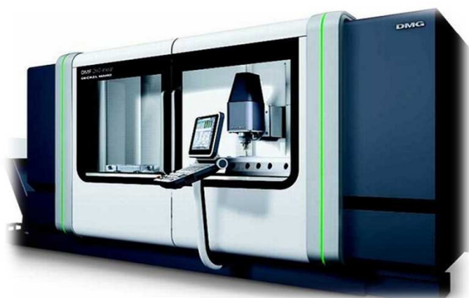
4 axis machining center Precision: 0.01 mm table: 2.9 m X 0.7 m
