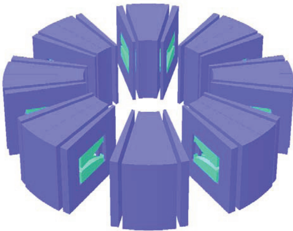
Figure 1: Magnet structure diagram without coils for eight super-periods.
