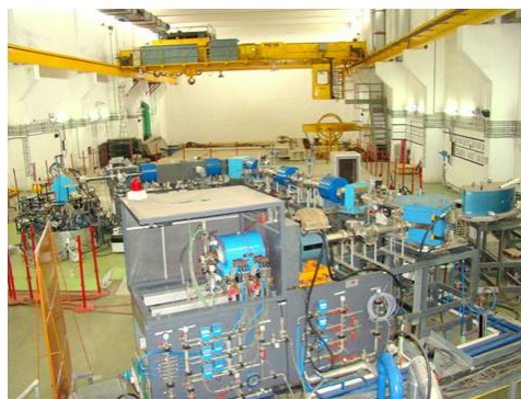
Figure 5: The ECR ion source and injection beam line in the high bay.
