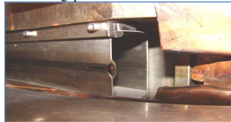
Figure 11: The first electrostatic deflector with 8mm gap between the electrode and septum.
