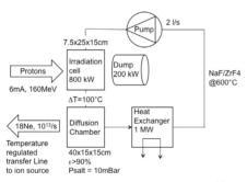
Figure 2: The molten salt loop to produce <sup>18</sup>Ne with an upgraded Linac 4 (CERN): 160MeV, 6 mA on average.
