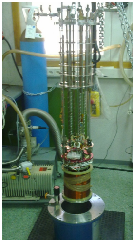
Figure 7: Prototype solenoids prepared for cold tests.
