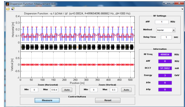
Figure 3: Dispersion function measurement GUI for the TPS storage ring.
