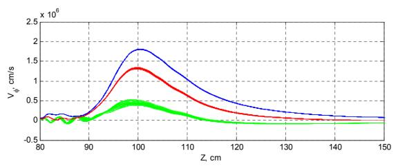
Figure 3: Azimuthal velocity of the antiprotons as a function of longitudinal position and at three different beam energies.
