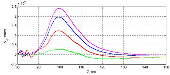
Figure 5:Azimuthal velocity of the antiprotons as function of the longitudinal position at different extraction energies: Green lines correspond to E=150 eV, red lines, 1,000eV, blue lines, 2,000eV, magenta, 3,000 eV. Magnetic field inside the trap B=5 T.
