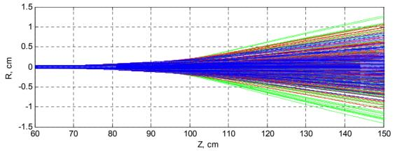
Figure 2: Particle trajectories. Blue lines correspond to an energy of E=150eV, green lines, E=1,000 eV, red lines, E=2,000 eV.
