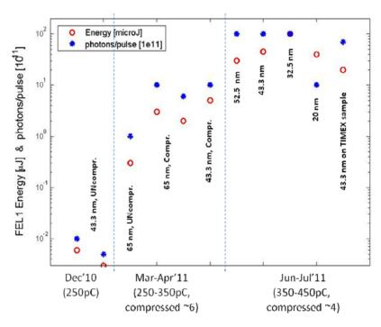
Figure 3: FEL-1 energy and photons per pulse during commissioning from December 2010 to July 2011.
