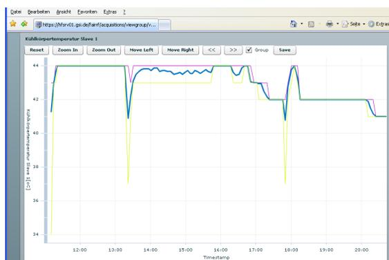
Figure 6 : Web interface: Data acquisitions; record of heat sink temperature of an RF driver temperature.
