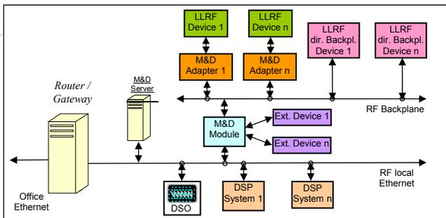
Figure 1 : Integration of different types of LLRF devices into the RF backplane standard.
