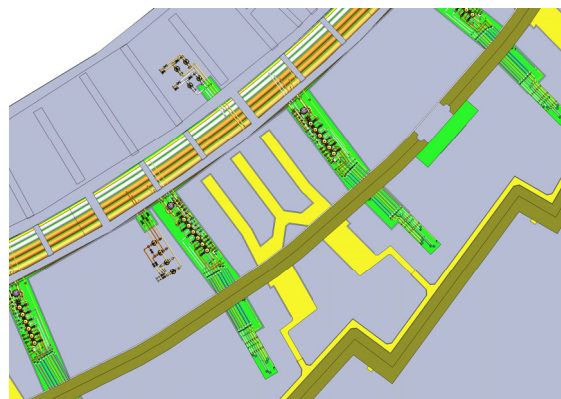
Figure 5: Manifolds for each section of the accelerator.
