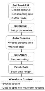
Figure 3: The EPICS record processing flow diagram for single data acquisition module.
