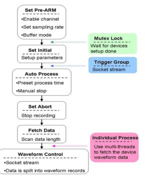
Figure 4: The EPICS record processing flow diagram for multiple data acquisition modules which are distributed nearby the measured area. Mutex Lock is used to avoid the race condition of device setup time. Trigger Group sends an UDP packet to trigger all modules to start recording.
