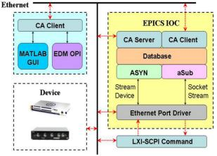
Figure 2: The block diagram of EPICS soft IOC which is communicated with the device via LXI-SCPI commands and Ethernet socket stream.
