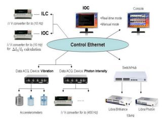
Figure 1: The structure of data acquisition system for vibration monitoring.
