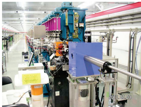
Figure 3: Installation of the HM that is covered with the geomagnetic shield box.
