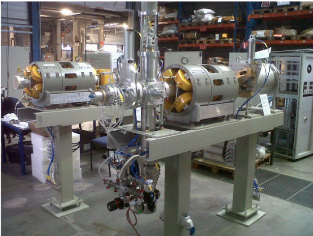
Figure 5: The external beam - assembled in Belgium - consists of two parts, one for each bunker. The quadrupole doublets and the neutron shutter are visible.
