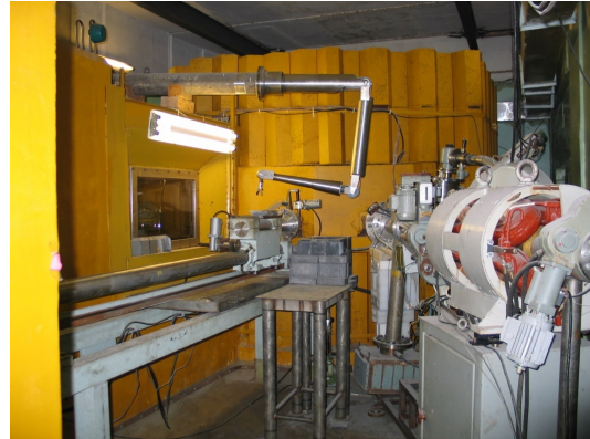
Figure 6: Isotope production installation (the proton beam magnets are at right hand).
