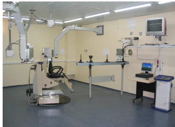
Figure 1: The first proton therapy treatment room (the entrance collimator is the circle at the right wall).
