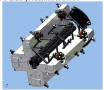
Figure 4: Cut-of the helical wiggler
