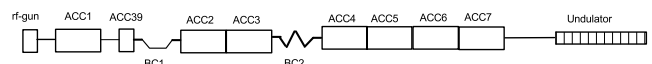
Figure 1: Schematic layout of the FLASH facility [3]. Abbreviations ACC1-ACC7, ACC39, and BC stand for accelerating module 1.3 GHz, accelerating module 3.9 GHz, and bunch compressor, respectively. Total length of the machine is 250 meters.
