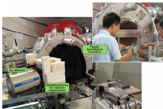
Figure 6: An illustration of the detector layout of the third MuSIC beam test in June, 2011.
