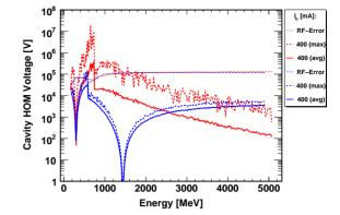
Figure 5: Average (solid) and maximum (dashed) cavity HOM voltages over the beam energy in the cavity centre. The maximum RF voltage error is indicated with dotted lines. The upper (red) curves are the BL layout and the lower (blue) the MS layout.
