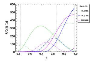
Figure 4:  $(R/Q)(\beta)$  plot of the TM<sub>010,4/5 $\pi$ </sub> (dashed) and TM<sub>010, $\pi$ </sub> (solid) modes. The entrance, transition, and output energy is indicated with vertical dotted lines.
