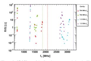
Figure 2:  $(R/Q)_{\text{max}}$  of the first three monopole bands. The dashed lines indicate the beam pipe cut-off frequency.
