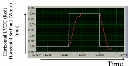
Figure 5: Backlash compensation strategy at positioning.
