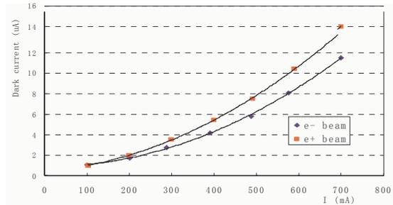
Figure 12: Dark current as a function of beam current.
