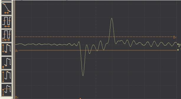
Figure 3: Single bunch measured with a BPM downstream the bunching system.
