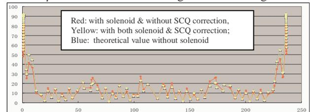
Figure 4: Vertical  $\beta$  function around the ring before and after the SCQ correction.
