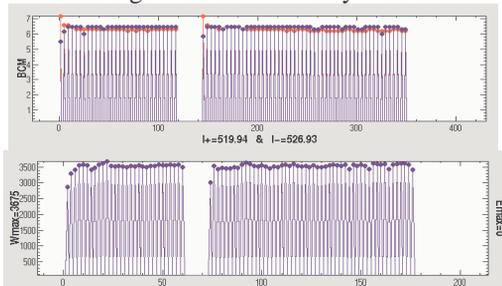
Figure 11: Bunch by bunch luminosity with longitudinal feedback system.(upper: bunch current, lower: luminosity)
