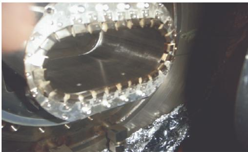
Figure 15: Damaged bellows and its RF fingers.
