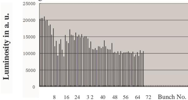
Figure 6: Bunch-by-bunch luminosity degrade along bunch train (same  $e^+$  &  $e^-$  bunch currents).
