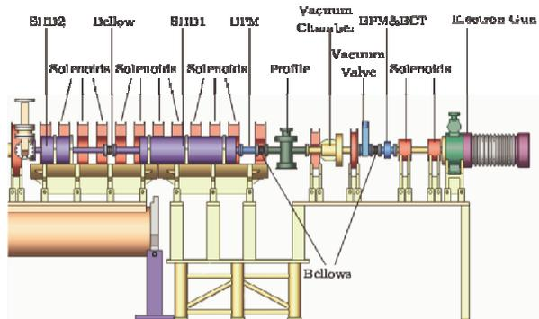
Figure 2: The front end of the BEPCII linac.
