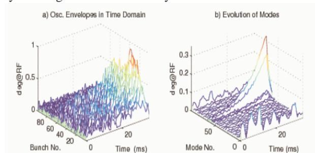
Figure 9: The instability mode of  $e^+$  beam in time domain.
