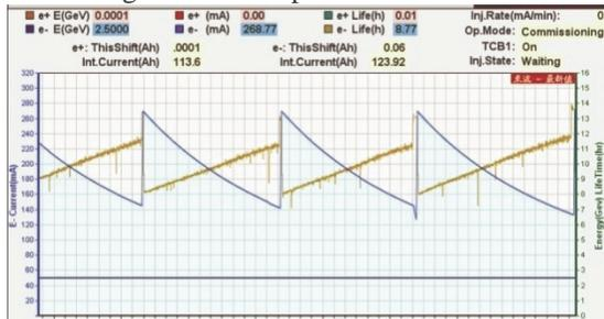
Figure 14: Typical beam current and lifetime during the routine operation for SR users.
