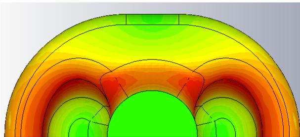
Figure 2: Absolute peak magnetic field of operating mode.
