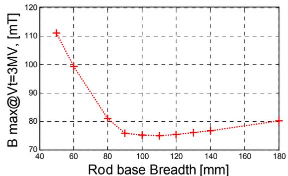
Figure 4: Peak magnetic field vs. rod base breadth.
