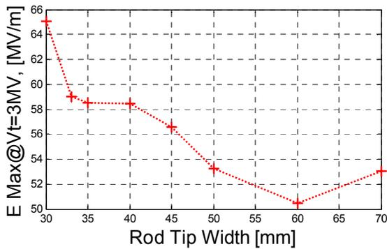
Figure 6: Peak electric field vs. rod tip width.
