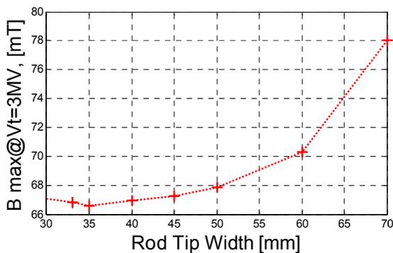
Figure 7: Peak magnetic field vs. rod tip breadth.
