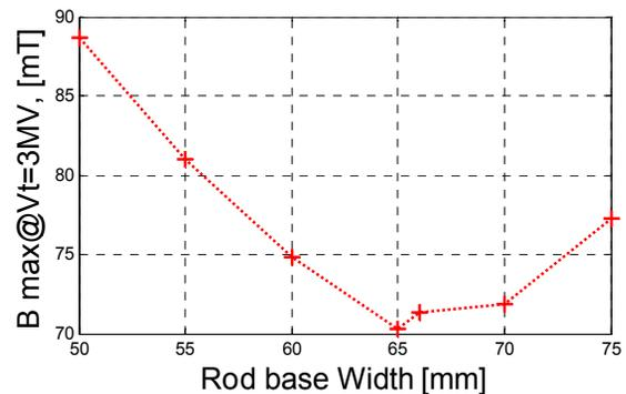
Figure 5: Peak magnetic field vs. Rod base width.
