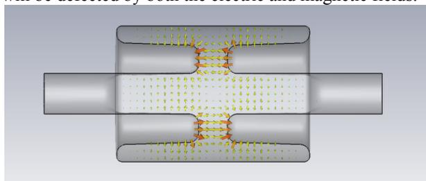
Figure 1: Electric field plot of cavity.
