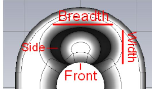
Figure 3: Descriptive terms used for the rod
