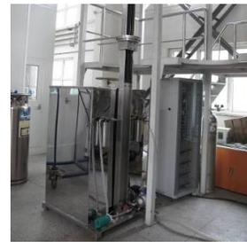
Figure 12: Ultrasonic cleaner for the 9-cell cavity
