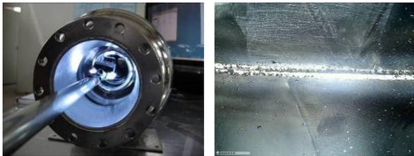
Figure 4: Inspection camera and the equator area of cell#2 as delivered
