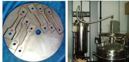
Figure 1: Large Grain Nb samples and test stand
