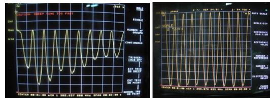
Figure 3: 9-cell cavity field flatness as delivered (70 %) and after pretuning (97.6 %)
