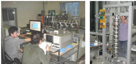
Figure 11: 9-cell cavity pretuning
