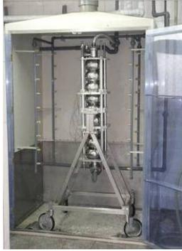
Figure 8: 9-cell cavity in the vertical CP facility
