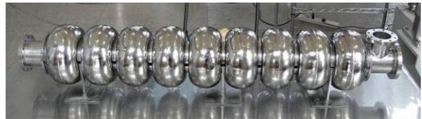
Figure 2: IHEP low-loss large grain 9-cell cavity
