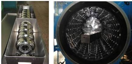
Figure 10: 9-cell cavity annealing
