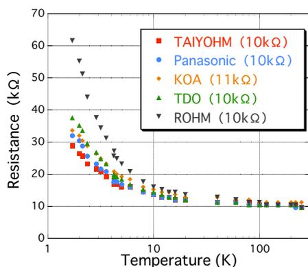
Figure 9: Plots of resistance values as a function of temperature for various manufacturers. The input current is 5 μA.
