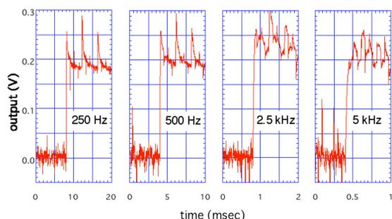
Figure 7: The output signal shape about difference of the switching speed (frequency).
