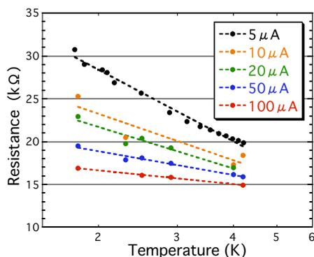
Figure 8: Plots of resistance value, as a function of temperature for various input current setting.
