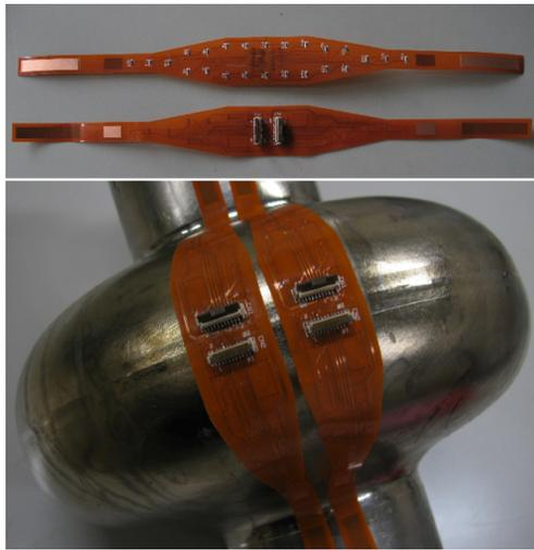
Figure 3: Experimental sensor strips. Resistors on flexible polyimide film contact with surface of Niobium cavity. In the final design of T-map system, the sensor assembly per sell consists of 32 strips (32 sensors per strip).
