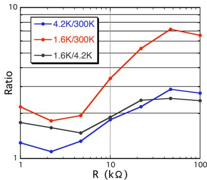
Figure 5: Sensitivity of Ruthenium oxide resistor.
