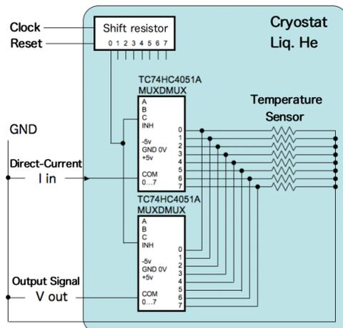
Figure 2: Test schematic diagram for T-map.
