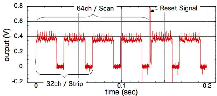
Figure 6: Output signal of experimental T-map system. 64 channels (12x4 sensors and 4x4 unused channels) are measured in one scan time. Temperature inside the cryostat, channel switching speed (frequency) and input current are 4 K, 250 Hz and 20 μA, respectively.
