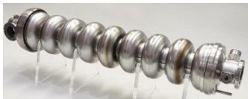
Figure 1: 9-sell superconducting accelerator cavity.
