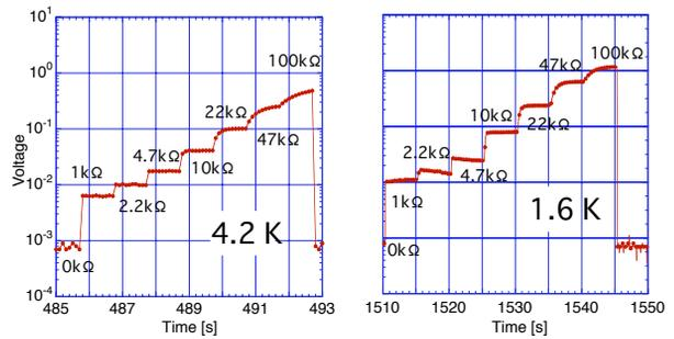
Figure 4: The output signals of Ruthenium oxide resistors. The left figure and the right were measured under cryogenic temperature of 4.2K and 1.6 K, respectively.
