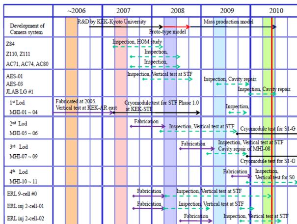
Figure 1: History of the inspection system and fabrication of the cavity.
