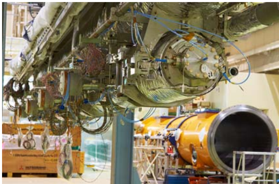
Figure 7: String cavities under the gas return pipe.
