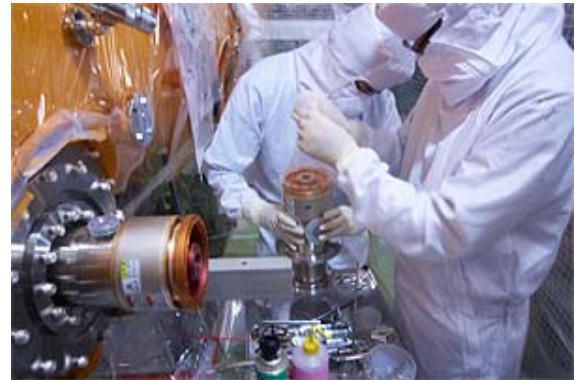
Figure 9: Assembly of warm parts for input couplers.
