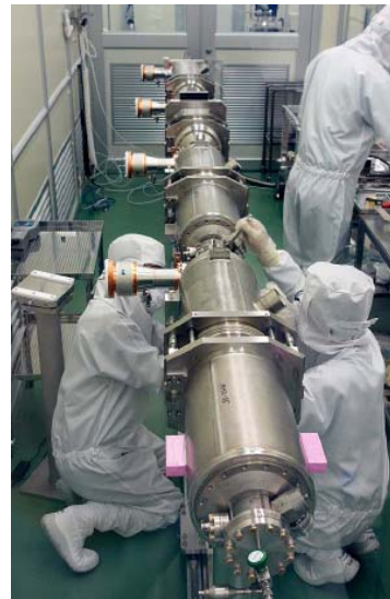
Figure 5: String assembly of four Tesla-like cavities.
