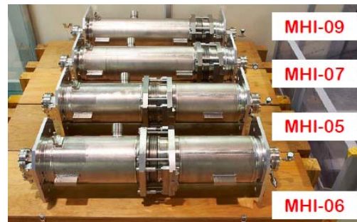
Figure 2: Four Tesla-like cavities for S1-Global.
