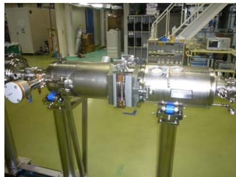
Figure 6: Attachment of a slide-jack and piezo tuner.
