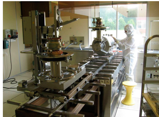
Figure 2: coupler assembly on the 5-cell cavity in the class 10 clean-room at Saclay/Orme des merisiers
