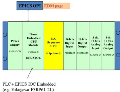
Figure 2: Configuration of EPICS PLC IOC for pulse magnet control.
