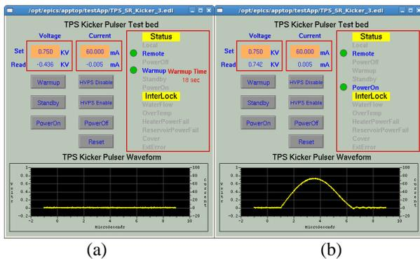
Figure 5: The control pages of pulse magnet power supply. (a) The thyatron tube warm up process in proceed. (b) High voltage power supply of kicker turn on and voltage sets 0.75 kV. The lower part of EDM page will display current waveform of kicker when trigger is active.
