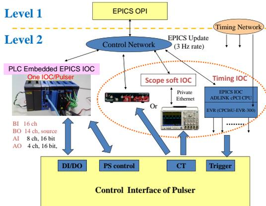
Figure 1: Control environment of the prototype pulse magnet power supply.
