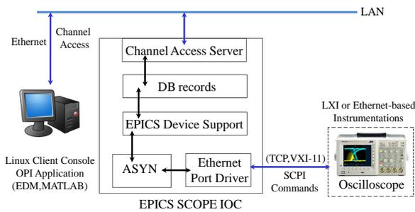
Figure 4: System architecture of building EPICS waveform support of LXI/Ethernet-based oscilloscope.
