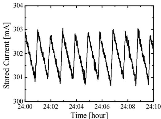
Figure 2: Time trend of beam current during a top-up operation.
