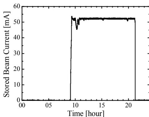
Figure 5: Single-bunch top-up operation in 9th, Sep. 2009.
