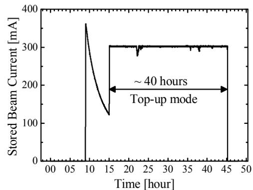
Figure 4: The 40-hour top-up operation in 4-5, Feb., 2010.
