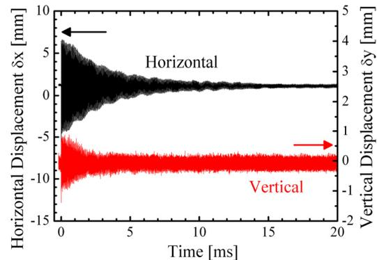
Figure 3: Beam orbit movement just after the injection measured at the entrance of the U5 in Fig. 1, outside of the injection bump.
