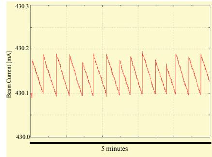
Figure 2: Five-minute record of top-up injections.
