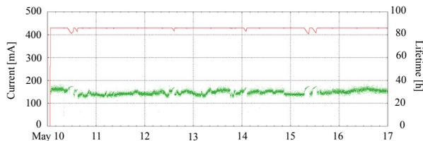
Figure 1: Record of the stored beam current (red line) and the beam lifetime (green dots) for seven consecutive days.
