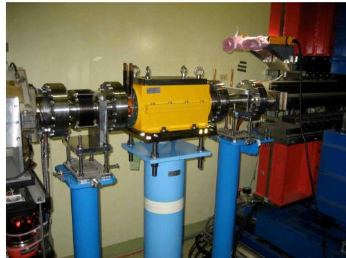
Figure 3: Pulsed sextupole magnet (yellow) installed in the PF-ring.
