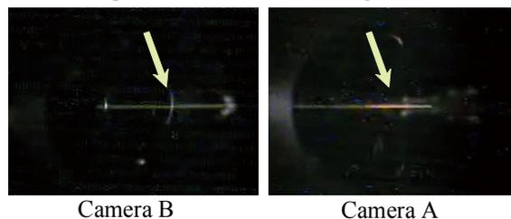
Figure 4: Trapped dust was visually observed using CCD cameras.
