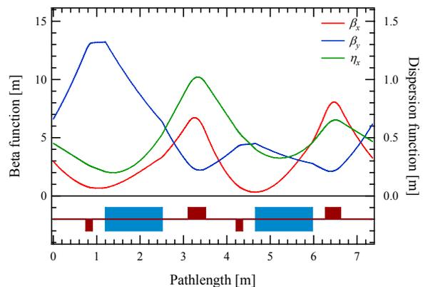
Figure 5: Optical functions of a booster ring
