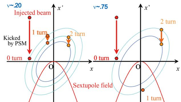
Figure 6: A behaviour of injected beam on phase space.
