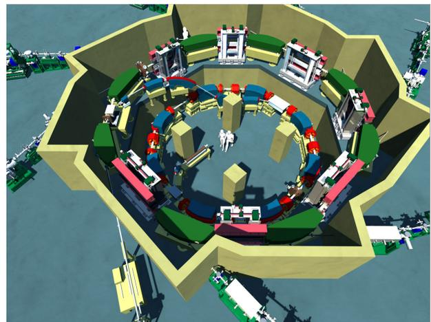
Figure 2: Layout of HiSOR-II storage ring and booster
