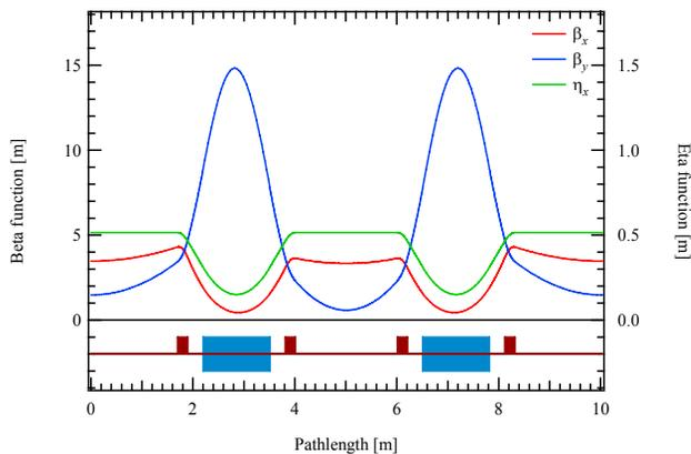
Figure 3: Optical functions of HiSOR-II storage ring
