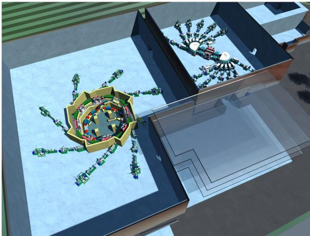
Figure 1: Layout of Accelerator complex of HSRC
