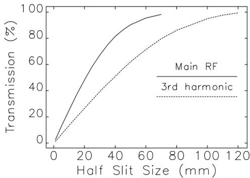
Figure 3. Transmission of the photons through the slit in the TPS photon beamline versus the half slit size, for the main and 3rd harmonic RF systems.
