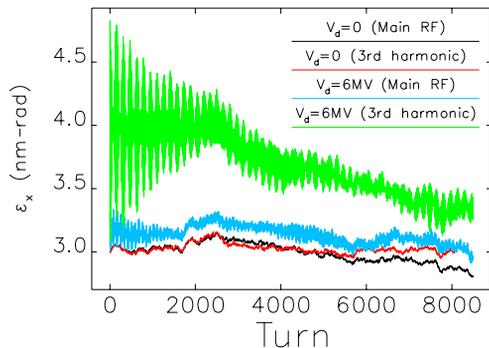
Figure 2(a): Horizontal emittance degradation on successive passes for the both main and 3rd harmonic RF systems in TPS.
