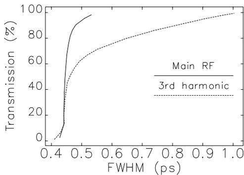
Figure 4. Transmission of the photons through the slit in the TPS photon beamline as a function of the FWHM of the X-ray pulses, for the main and 3rd harmonic RF systems.
