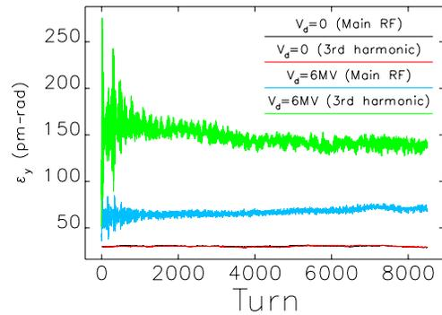
Figure 2(b): Vertical emittance degradation on successive passes for the both main and 3rd harmonic RF systems in TPS.
