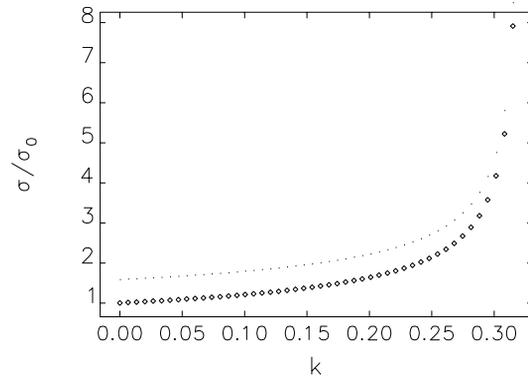
Figure 1. The normalized bunch length as a function of  $k$  for the third harmonic RF system in TPS. The main RF gap voltage is fixed at 3 MV ( $\varphi_s=163.66$ ,  $\varphi_n=358.14$  degrees and  $E=3$  GeV).
