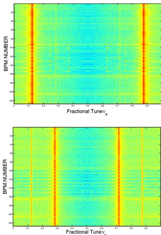
Figure 1: Colour plot of the FFT of the signal acquired at all BPMs after a combined horizontal and vertical kick of  $\varepsilon_x = 1.225$  mm mrad and  $\varepsilon_y = 0.85$  mm mrad. The horizontal (vertical) spectrum is shown in the upper (lower) plot.
