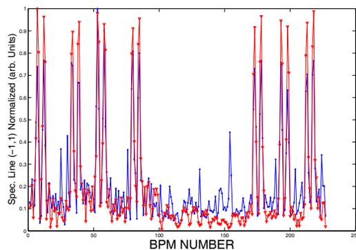
Figure 4: Longitudinal variation of the spectral line (-1,1) excited in the vertical plane: blue is measured, the red curve is obtained from tracking with SixTrack.
