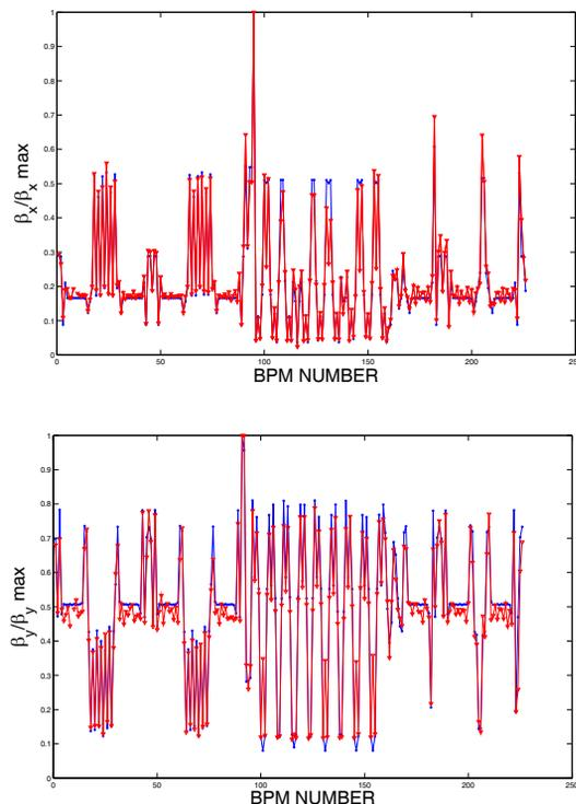
Figure 2: Comparison of the beta functions from the square of the the amplitude of the tune spectral lines (red) and from the MadX model (blue).
