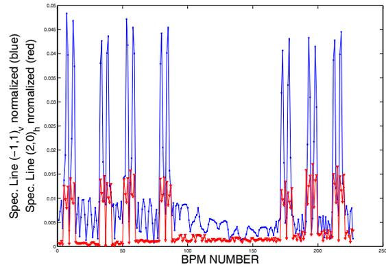
Figure 5: Comparison of the amplitude of the spectral lines (-1,1)(blue) in the vertical plane and (2,0)(red) in the horizontal plane derived from tracking data. Both lines are normalized to the tune lines.
