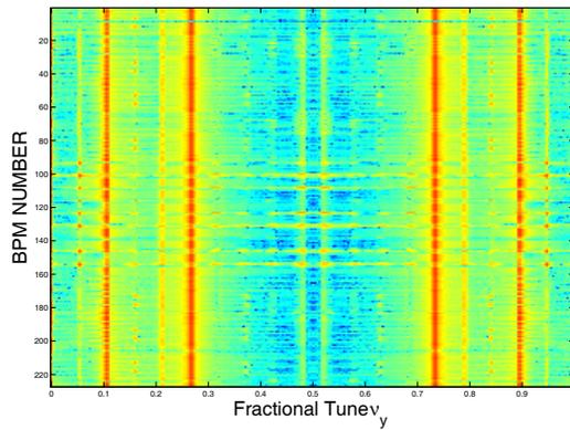
Figure 3: Colour plot of the FFT of the vertical signal acquired at all BPMs after a combined large horizontal and vertical kick of  $\varepsilon_x = 15$  mm mrad and  $\varepsilon_y = 0.4$  mm mrad, respectively.
