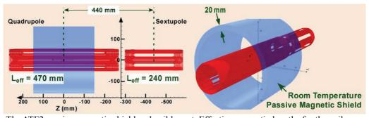
Figure 3: The ATF2 passive magnetic shield and coil layout. Effective magnetic lengths for the coils are as shown. shows schematically how the quadrupole was wound in three coil sets for a total of six cable layers.
