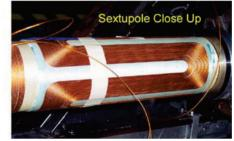
windings on a shared support tube [2]. The coils are wound as multi-layer Serpentine style coil patterns using computer controlled Direct Wind technology developed at BNL [3]. The quad and sextupole coil patterns, formed from seven-strand round (about 1 mm diameter) cable, are shown in Figure 1. The sextupole coil was wound in two Serpentine coil sets (four lavers total). Figure 2
