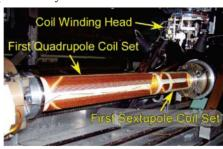
Figure 1: Start of ATF2 main quadrupole and sextupole Serpentine style coil winding.
