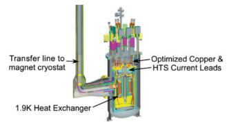
Figure 6: Cutaway View of the ILC Service Cryostat.
