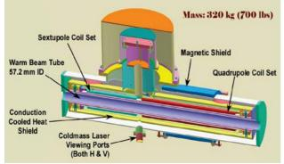
Figure 4: Magnet cryostat design features (as indicated). 03 Linear Colliders, Lepton Accelerators and New Acceleration Techniques
