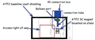
Figure 7: ATF2 SC Magnet with 4K Connection Box
