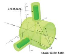
Figure 5: Magnetic shield design now has laser access to the magnetic center of the quadrupole coil. Four holes were created to maintain quad symmetry (only two used for lasers). Additional shielding around the Geophones counters local field spikes near the other penetrations.
