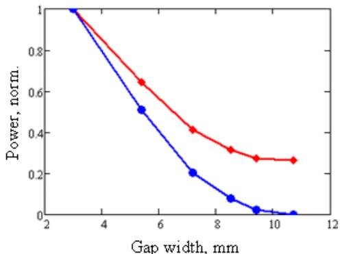
Figure 11: Normalized steady state rf power levels at the structure input (blue) and the PETS output (red) for the different piston positions.
