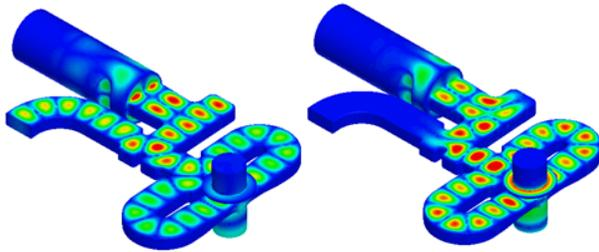
Figure 3: Electric field plots for the reflector in ON (left) and in OFF (right) positions.
