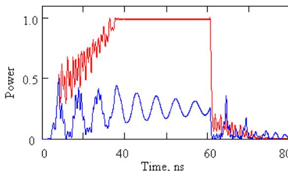
Figure 2: RF pulses envelopes at the PETS output for the ON (red) and OFF (blue) positions of the reflector.
