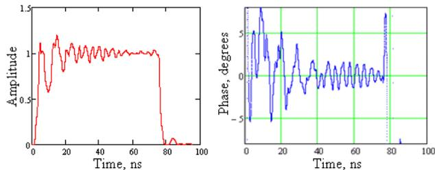
Figure 4: The generated rf pulse envelope (left) and rf phase profile (right) for the reflector in ON position.
