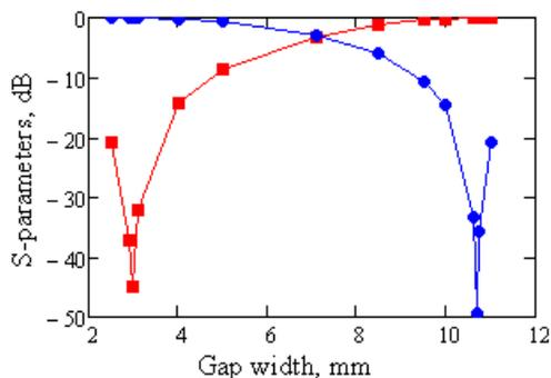
Figure 9: Reflection (red) and transmission (blue) for the different position of the piston at 12 GHz.
