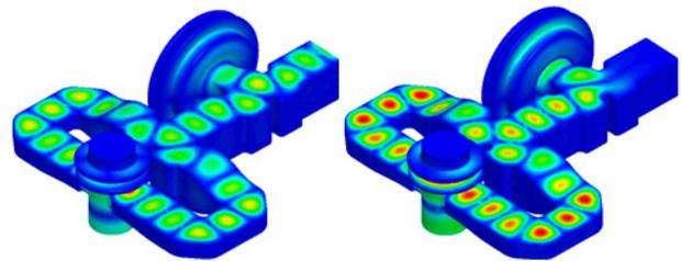
Figure 7: Electric field plots for the reflector in ON (left) and in OFF (right) positions.
