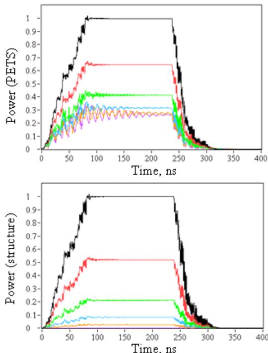
Figure 10: RF pulses envelopes at the PETS output (top) and the structure input (bottom). Here the reducing amplitudes correspond to the different piston positions.
