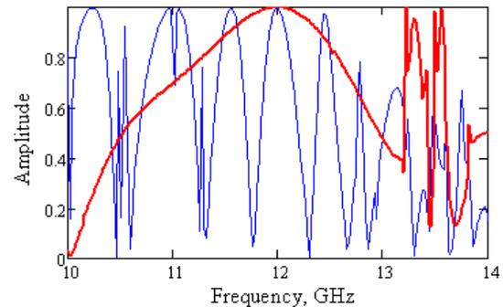
Figure 6: Transmission of the reflector in ON position. Here in blue is for the first reflector version and in red is for the new design.
