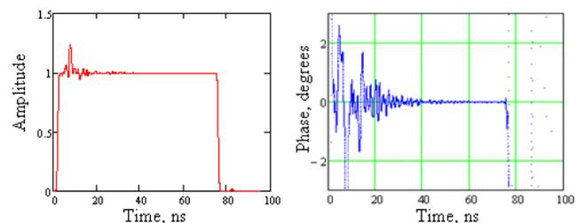
Figure 8: The generated rf pulse envelope (left) and rf phase profile (right) for the reflector in ON position.
