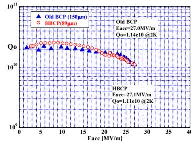
Figure 9: Vertical test results on I9#9.
