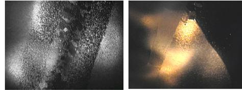
Figure 8: Different metallography seen at the EBW seam between fine (left) and large grain (right) Nb materials.
