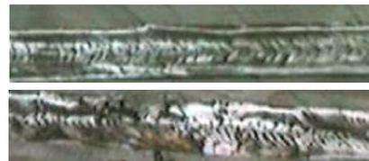
Figure 5: Equator EBW seams of I9#10 cavity. Top is most stable one and bottom is most unstable one.
