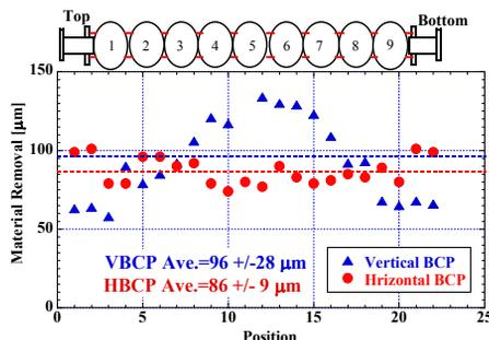
Figure 7: Comparison of material removal between the old and HBCP methods.
