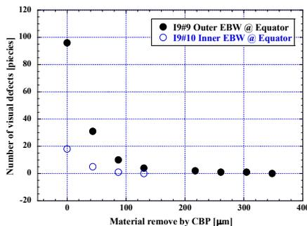
Figure 6: Comparison of defect distribution on the surface between inner and outer EBWs.
