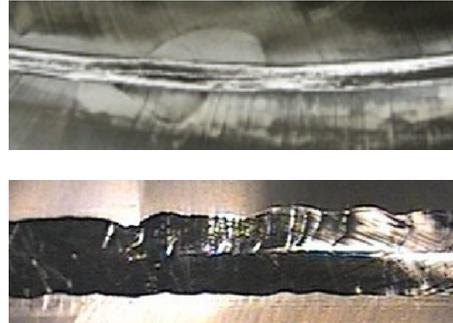
Figure 4: Comparison of EBW seams between the inner (top) and outer (bottom) EBWs at equators on large grain cavity.
