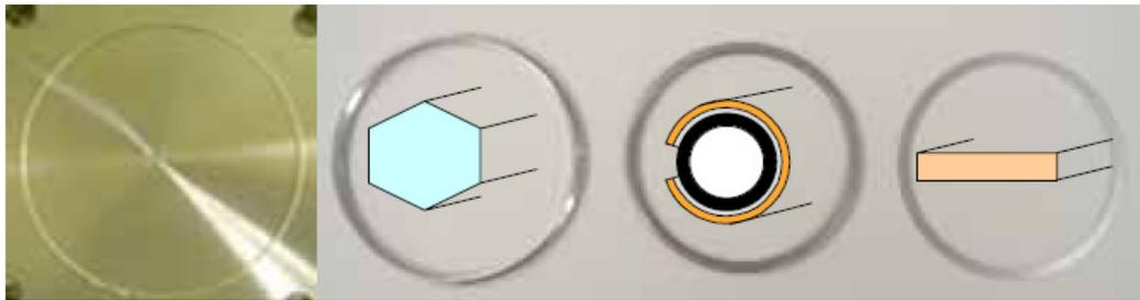
Indium wire sealing    DESY “Diamond gasket”    In plated U-tight seal    MO seal (Al or Cu)
