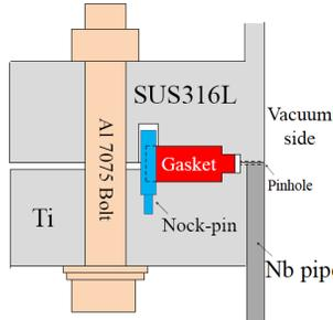
Fig.3: Modified MO flange. The size is not scaled.
