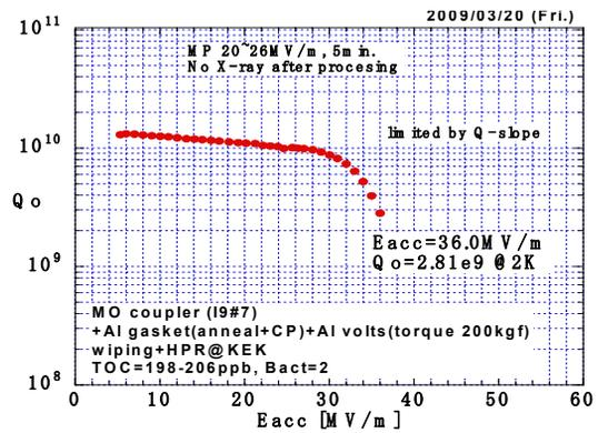
Fig.7: An example of successful vertical test using MO seal.
