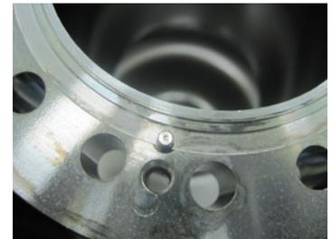
Fig.8: Titanium flange corrosion during BCP
