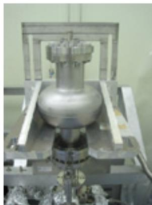
Fig.6: MO seal test with single cell cavity.
