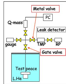
Fig.4: High sensitive cold leak test system at KEK
