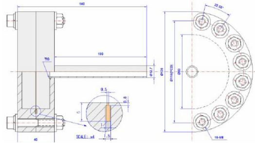
Fig.1 The Original MO seal design by H.Matsumoto. currently used in SRF field. The feature 2) looks like the ICF seal, which has a knife-edge but has a gap between flanges. MO seal is better structure for RF shielding than ICF design.
