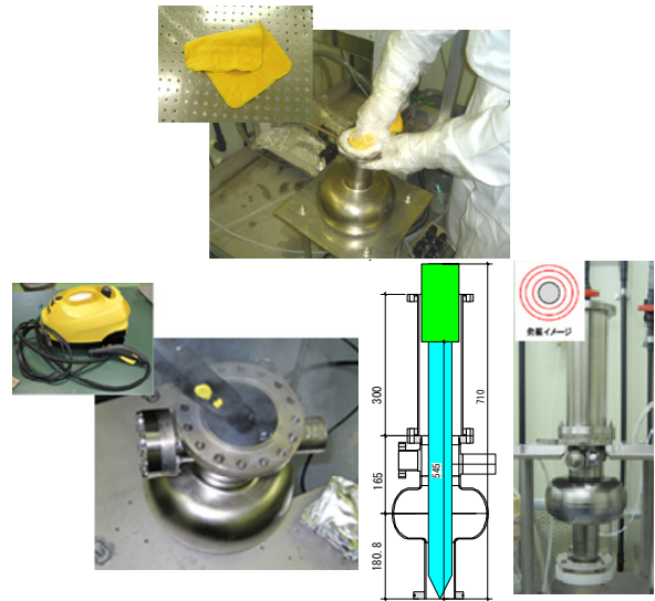
Figure 4: post EP cleaning, Top: Wiping, Bottom left: Steam cleaning, Bottom right: Horn rinsing
