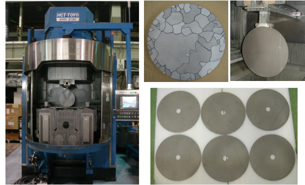
Figure 2: slicing machine, sliced Nb sheets.
