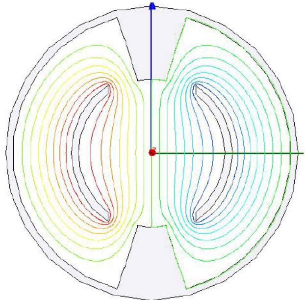
Figure 1. Cross section of magnet and flux lines.
