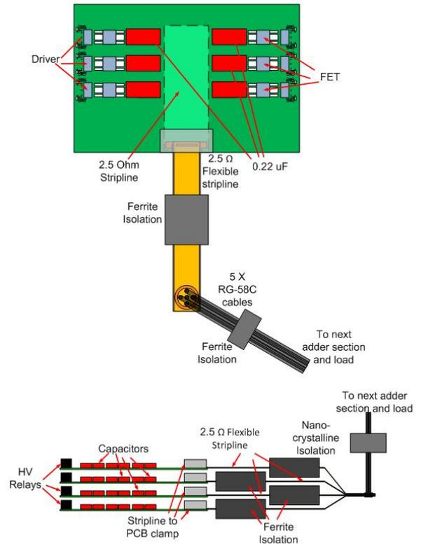
Figure 4. Drawing of the switch PCBs and adders.
