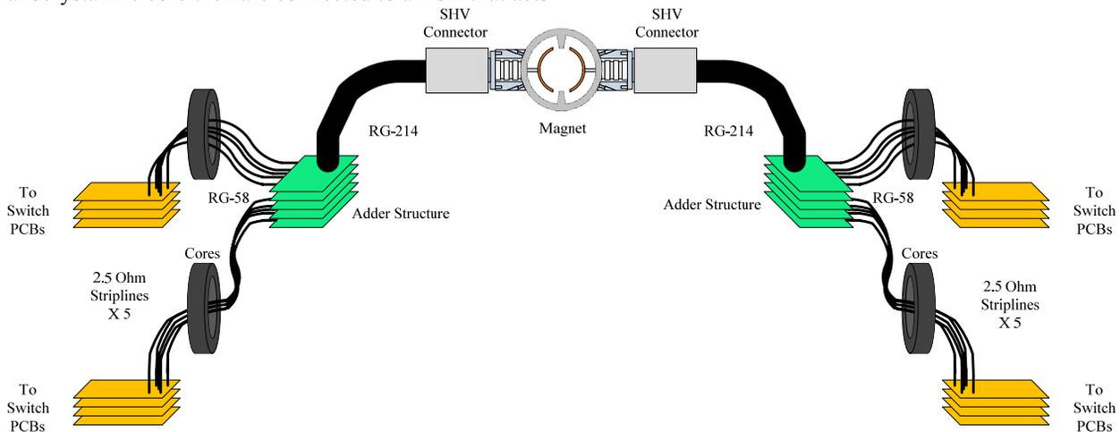
Figure 5. Drawing of assembled transmission line adder.
