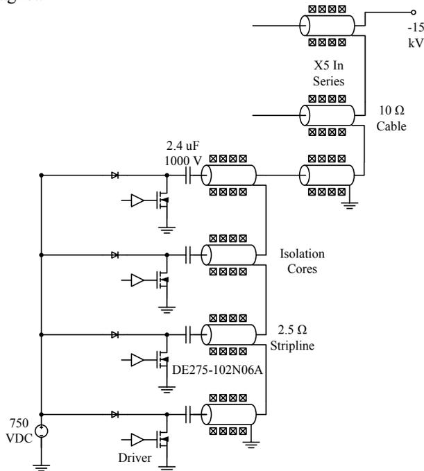
Figure 3. Simplified schematic of a transmission line adder.
