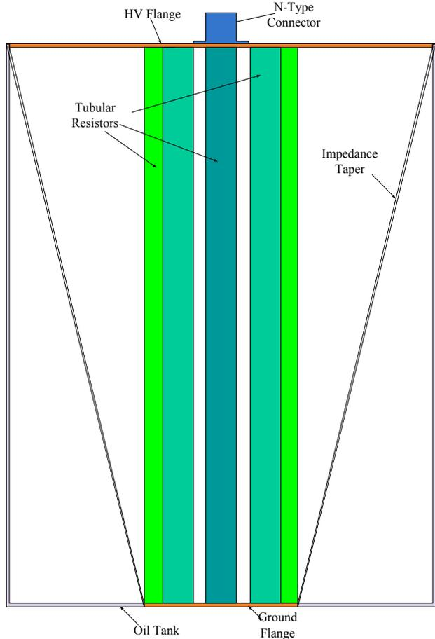
Figure 6. Drawing of the resistive load.
