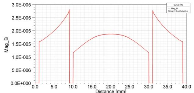
Figure 2. B field magnitude across center of aperture.
