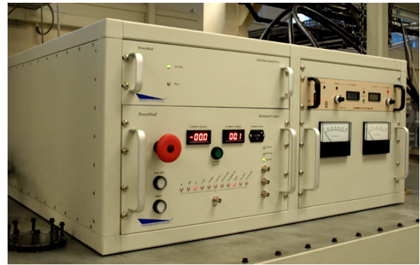
Figure 5: Modulator Controls, including fast fault detection and first fault identification.
