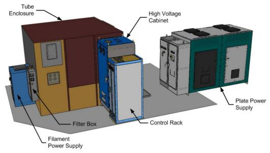
Figure 2: Tetrode test stand assembly.
