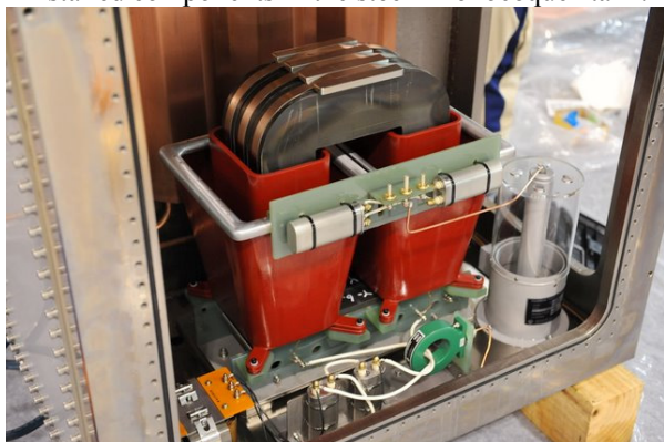
Pulse transformer using epoxy molded windings and low loss Super-E core.
