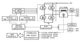
Figure 2: The structure of corrector power converter
