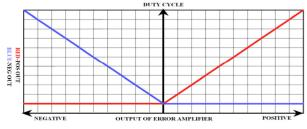
Figure 3: The relationship between the switching duty cycles and the output of error amplifier
